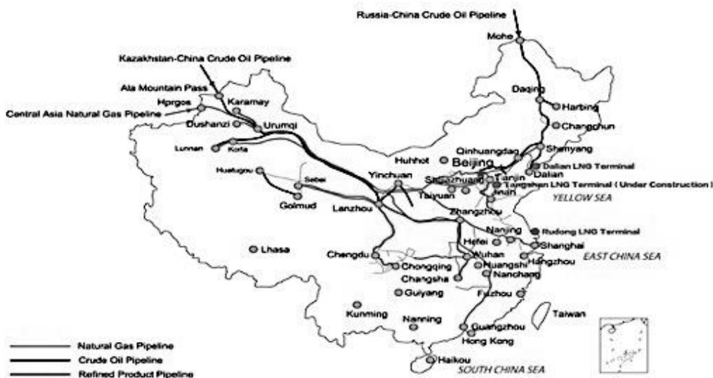
Diagram 2 — Main gas and oil pipelines in China
